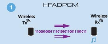
A narrow signal band is used that is sufficient enough for high-quality audio transmission yet perfect for finding a path through the congested environment of a home filled with potentially conflicting devices. This narrow band is a feature of HFADPCM (High Fidelity Adaptive Differential Pulse Code Modulation), and along with advanced error correction technology ensures an exceptionally robust delivery of CD-quality audio between the transmitter and receivers.
